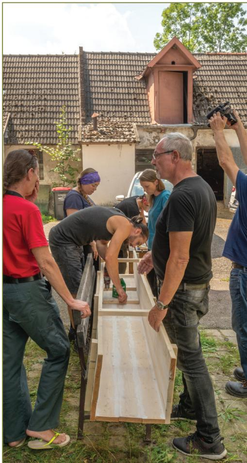
**Fig 5.** Attaching the wooden strips to the bottom of the sluice-box. Photo by F. Stremke
