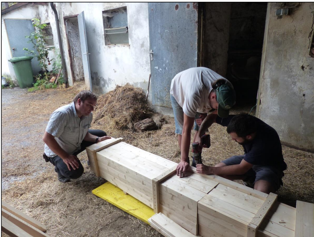
Fig 13. Joining the two halves of the sluice-box. Photo by B. Cech
