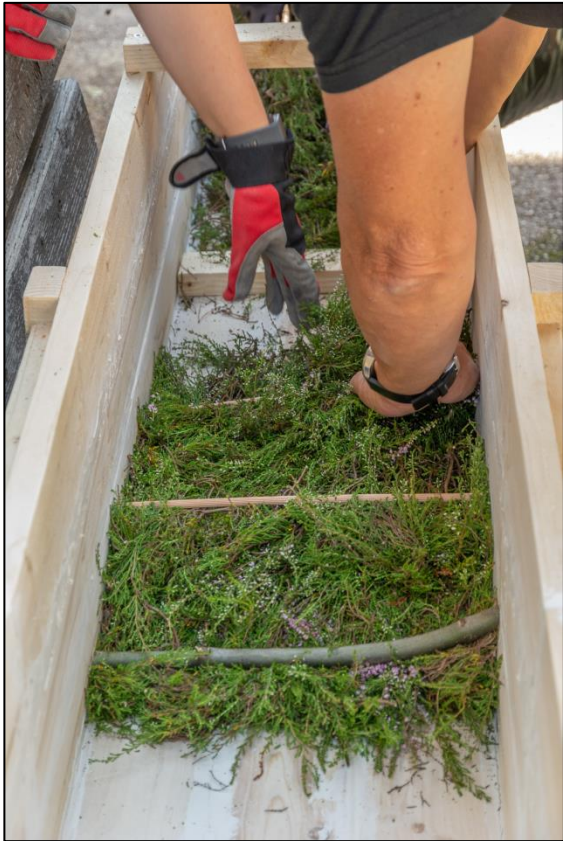
Fig 17. Lining the bottom of the sluice-box with heather and fixing it with thin wooden strips and twigs. Photo by F. Stremke
