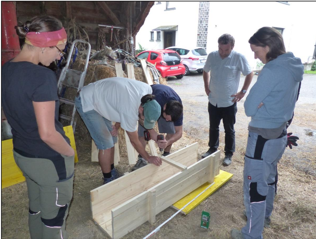
Fig 12. Attaching the struts to one half of the sluice-box. Photo by B. Cech
