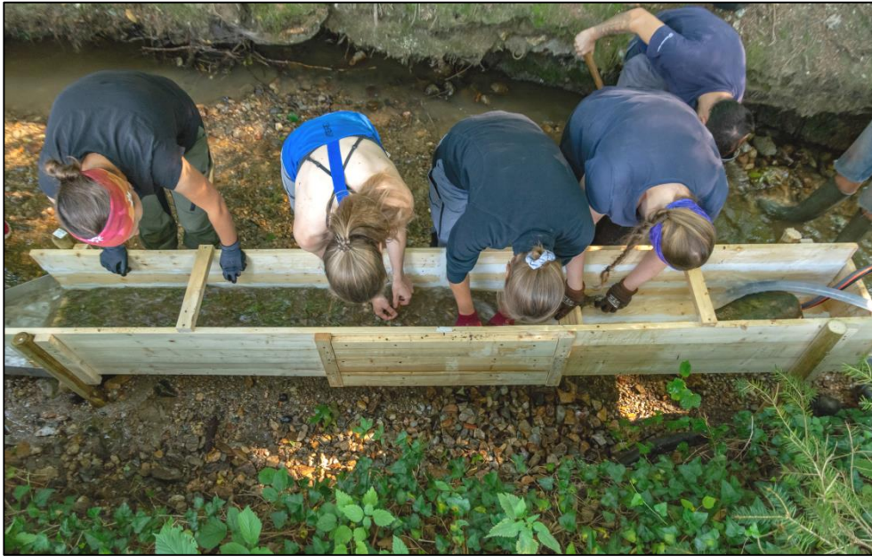
Fig 21. Keeping the sediment in constant movement while removing stones. Photo by F. Stremke
