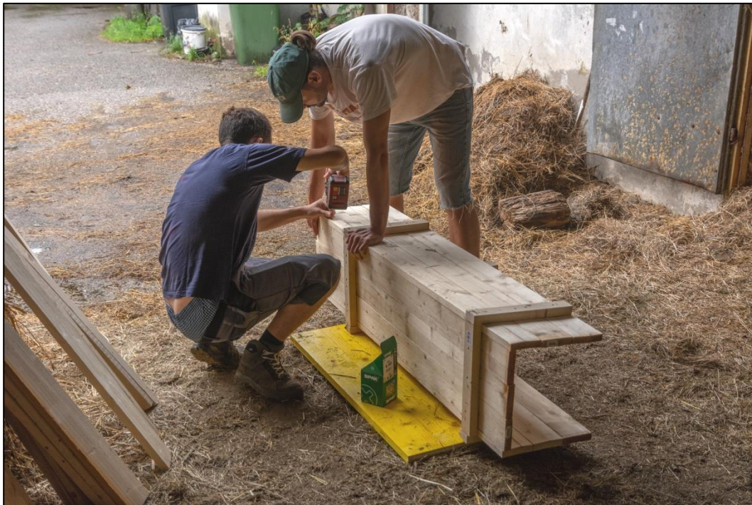
Fig 11. Assembling one half of the sluice-box . Photo by F. Stremke
