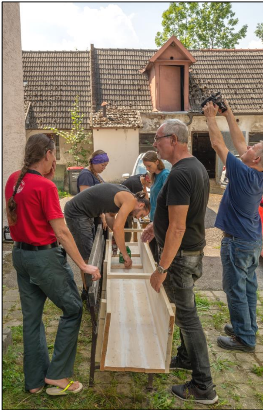
Fig 14. Attaching the wooden strips to the bottom of the sluice-box. Photo by F. Stremke
