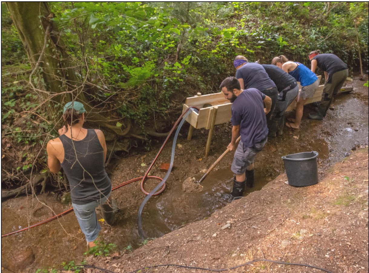
Fig 20. The reconstructed sluice-box in operation. Photo by F. Stremke
